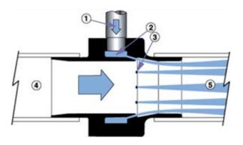
Compressed air flows through the inlet (1) into an annular plenum chamber (2). It is then injected into the throat through directed nozzles (3). These jets of air create a vacuum at the intake (4) which draws material in and accelerates it through the unit (5) for conveying over long vertical or horizontal distances.
