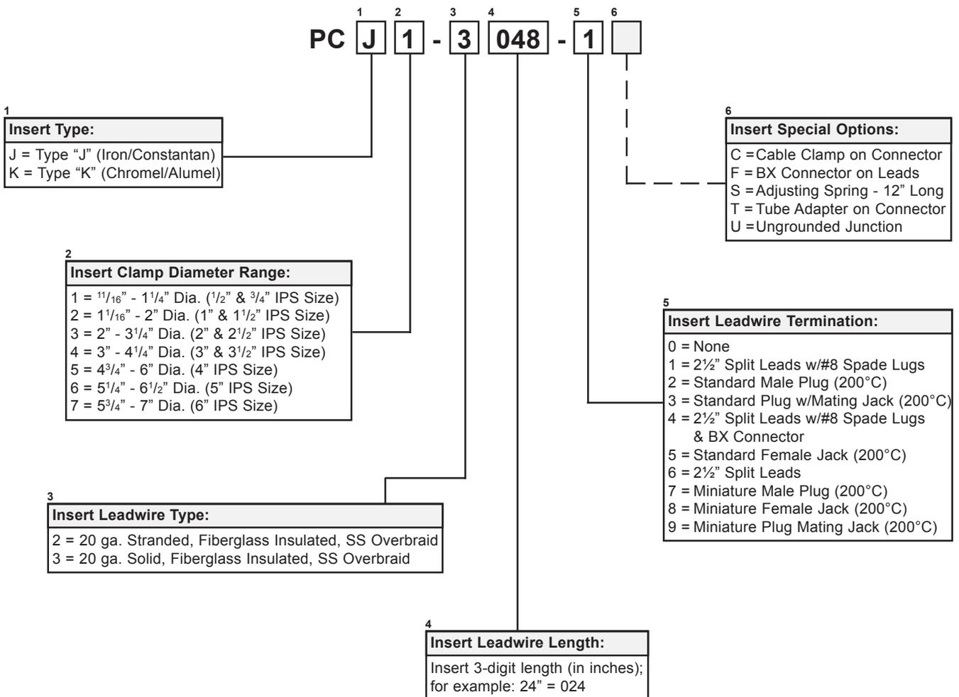
**Ungrounded also available. (For Ungrounded, MgO insulation will be provided for better isolation of temperature sensing element.)**
